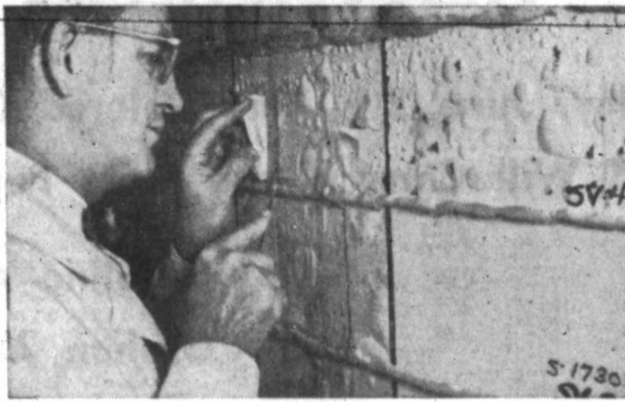
Laboratory Blister-Test shows how regular house paints react to abnormal moisture conditions, compared to "Lucite" over Du Pont Blister-Resistant Primer (lower right panel), which shows no sign of blistering.
