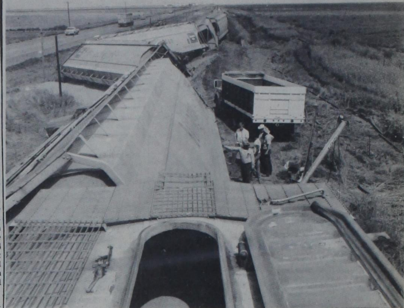
GRAIN CARS DERAILED —Five grain gondolas of the Fort Worth & Dancer Railroad, loaded with wheat from Dimmitt elevators, jumped the track west of Hart Wednesday afternoon. This photo, taken from atop a car still on the track, shows how the mid-train cars jack-knifed, throwing one car onto its side and ripping off its wheel assemblies. The force of the derailment rip-
