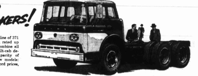
New additions to Ford's '59 line of 371 models—Tilt Cab Tandems, rated up to 75,000-lb. GCW! They combine all the advantages of modern tilt-cab design with the carrying capacity of tandem axles. Other all-new models: 4-wheel drive units at low Ford prices, available early in 1959.
