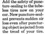
The most recent technological advance from United States Rubber's Research Laboratories is a "weightless sealant" called AIR GUARD. This sealant, when placed in tubeless tires, ends the danger of roadside tire changing due to
