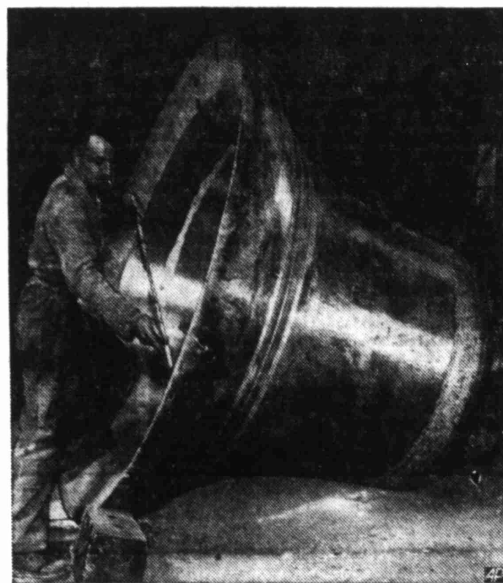
FOUNDRY CHECK — Worker sizes six-ton bell, largest of set prepared at Ancey, France, for the Robert A. Taft Memorial Monument in Washington, D.C., will be 100 feet high.
