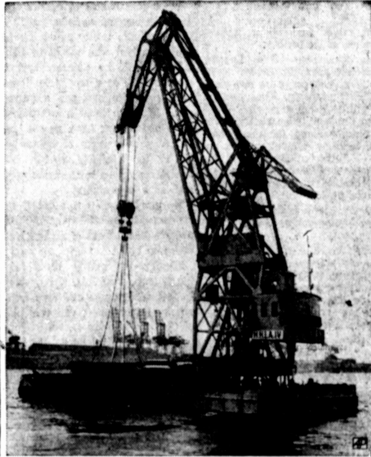
FLOATING POWER — Germany's largest "floating" crane goes to work in Hamburg harbor. The new hoist is powered by a 515-hp diesel engine and has a lifting power of 200 tons.
