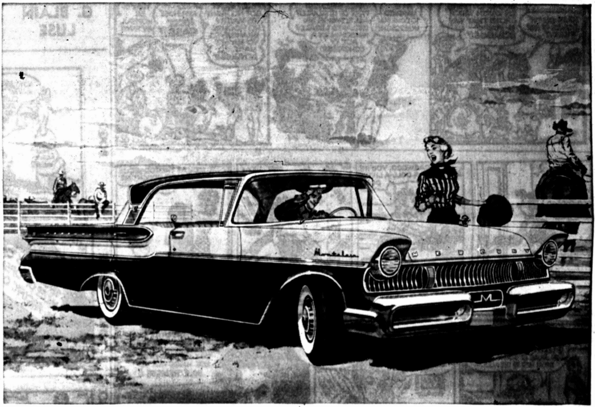
YOU ENJOY INCREASED HEADROOM...made possible by recessing the floor within the frame, and by the unique, straight-line design of the roof. Mercury's outside height is a sleek, shoulder-high 4 feet 8 inches.
