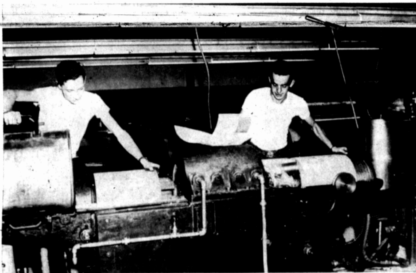
PLATES FOR PRESS ARE CAST NEXT Pressman Leon Tate, Stereotyper Roy Dirickson operate plate making machine.
