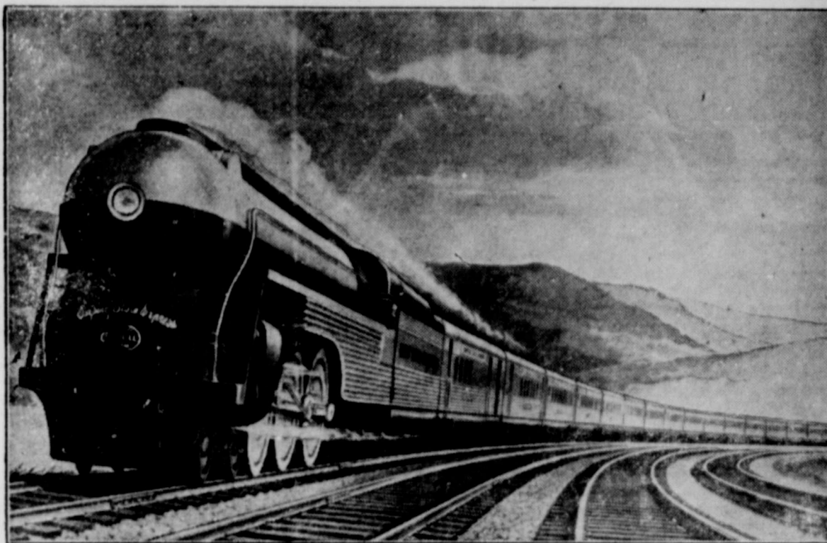
FIRST picture of the new Empire State Express, New York Central's new super-streamliner to be placed in service within a few weeks between New York, Buffalo, Cleveland and Detroit. Its 32 stainless steel cars are now nearing completion in the Philadelphia shops of the Edward G. Budd Manufacturing Company, while its streamlined Hudson locomotives will soon be completed by the New York Central's shops. Hailed as the world's most modern day train, it will be operated each way daily in two sections of 13 to 16 cars each.
