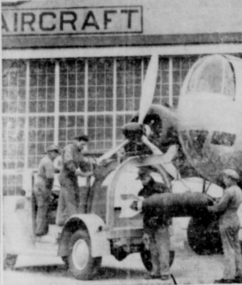
SELFLEDGE FIELD, Mich.—A familiar piece of motorized equipment around U. S. Army Air Corps bases these days is this service truck, shown being operated near a big dummy bomb at Selfledge Field. Manufactured by the Ford Motor Company, the truck is rigged with special derrick and windlass to handle bombs weighing 600 to 1,200 pounds. The bomb in the photo is a dummy 600-pounder used for training purposes.
