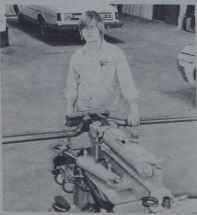
PRECISION BENDING —Gary Williams uses our new Huth pipe bender to make a customized 2-inch tailpipe for a Chevrolet pickup.
