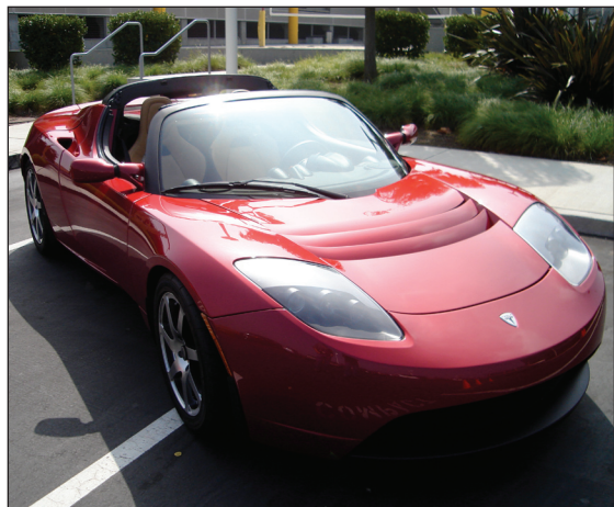
The Tesla Roadster, an electric sports car with a huge battery, can draw 16,800 watts. That's the equivalent of 280 60-watt light bulbs.
