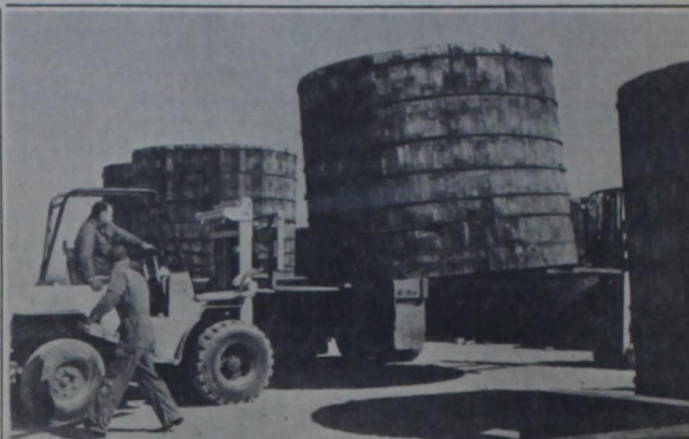
EASY, NOW —Front loaders ease a big wooden brine tank to the ground after lifting it from a truck bed so the truck could be driven out from under it at the Western Vegetables cucumber processing plant.
