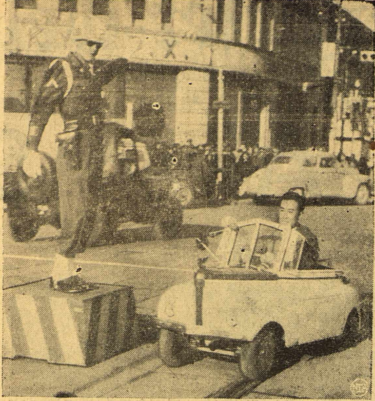
Yoshiharu Yamanaka beams as he takes his midget electric car along a Tokyo street, startling an American MP on traffic duty. The tiny vehicle has a 400-watt motor developing one-half horsepower, enabling it to run for three hours at 25 miles an hour. Wheels are taken from dismantled airplanes.
