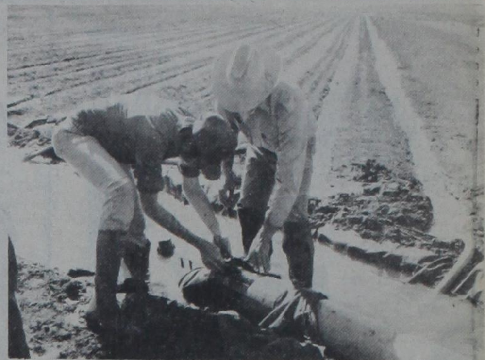
Gary Hunter, Soil Conservationist at Dimmitt, assists Rayphard Smithson in checking the gallons per minute his wells are producing. These wells were checked with the District owned Sparling Flow Meter. The services of this equipment is provided to anyone in the Running Water SWCD, at no charge. The District Directors feel that the information provided is a must for local producers in the battle of reducing the cost of irrigation.
