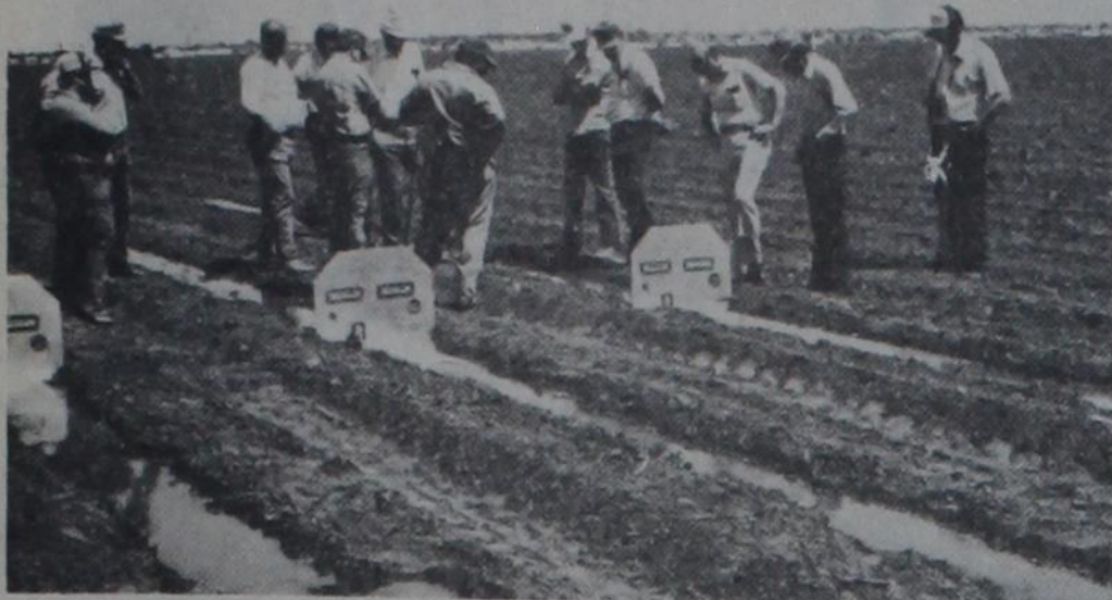
The Running Water SWCD and SCS are making consolidated efforts this summer to gather data to help improve irrigation water management. One method of obtaining this information is doing a series of furrow evaluations to determine the intake efficiency of the soils in Castro County. Oriface Plates are set in rows at the top and lower ends of the field. The use of these plates enables the SCS Technicians to record the actual amount of water being absorbed by the soil. This information will be used to design proper irrigation systems.
