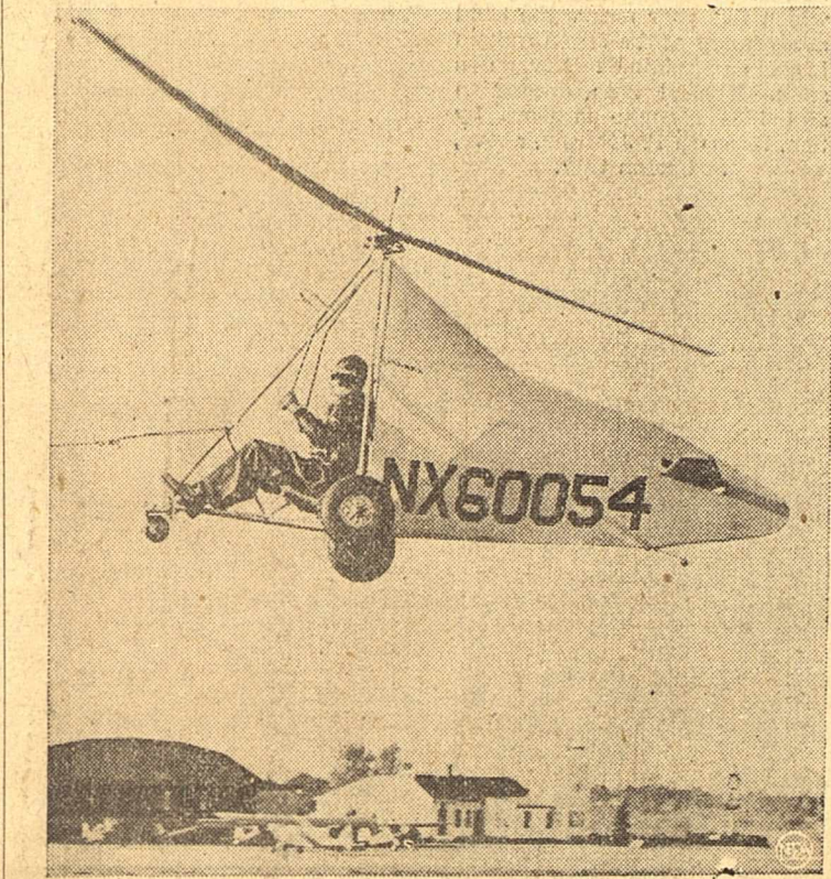
Queer-looking craft above is a new wingless glider, known as the G-E Gyro-Glider, pictured during recent test run, towed by a jeep, at Schenectady, N. Y. Glider, which works like a motorless autogyro, is reported, capable of lifting nearly 300 pounds in addition to its own weight and can land in extremely small space.
