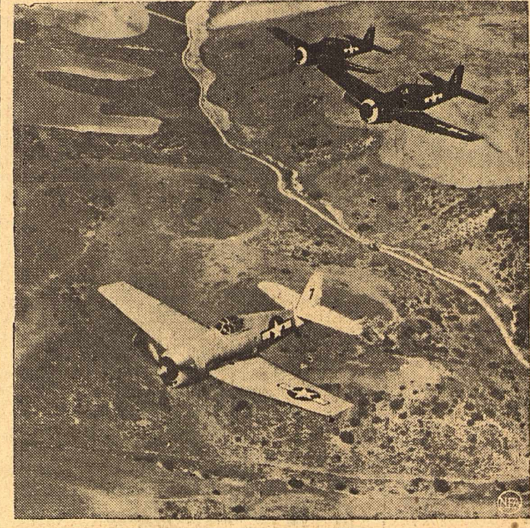
Hellcat drone in lead is controlled by "queen" or mother Hellcat directly behind it. Second control plane stands by in case of failure in first one.
