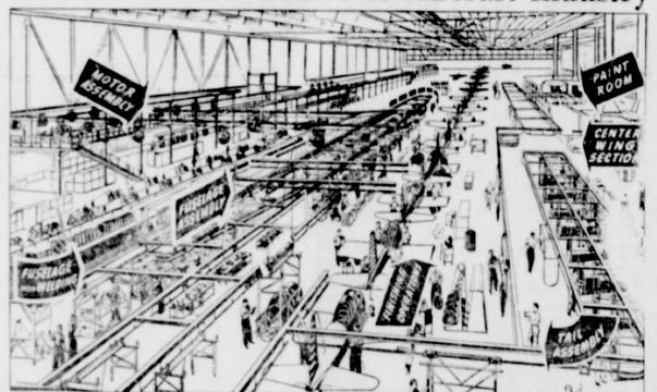
The above drawing of Vultee | bring all five together at the nerve | production developments at the the plane ready for flight. California plant in the last few At the right of the picture, tail mount and attaching controls, pipmonths. It is the graphic story sections are assembled, complete ing and other "plumbing." A of how modern airplanes are with monocoque, stabilizers, rud- chain-driven overhead conveyor n the aircraft industry.
