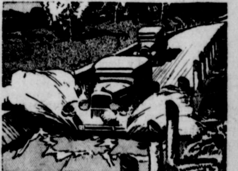
A scientific "bath tub"—not to wash cars, but to show the Proving Ground engineers exactly what happens when a car is driven through water.
