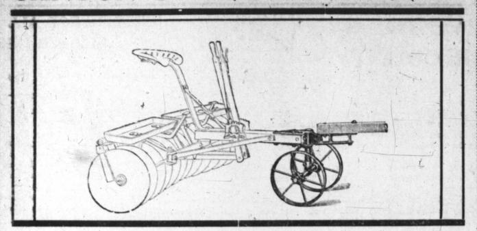
In sizes 6, 7 and 9 foot with tongue trucks, will run steady as a wagon and without any side draft or neck weight. Easy to handle. We also have the tandum attachment for this harrow, which can be attached behind, double discing your land as you go, one man doing the work of two. This harrow is equipped with hard wood maple bearings, making it the longest lift harrow on the market. This harrow has no equal. Come let us show you this up-to-date harrow.
