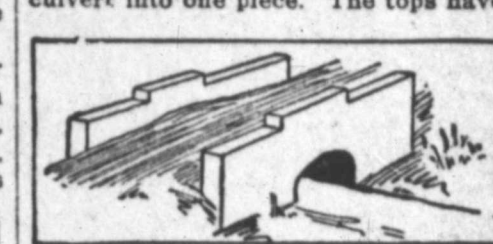
Flat-Top Style of Culvert an Approved Type.
