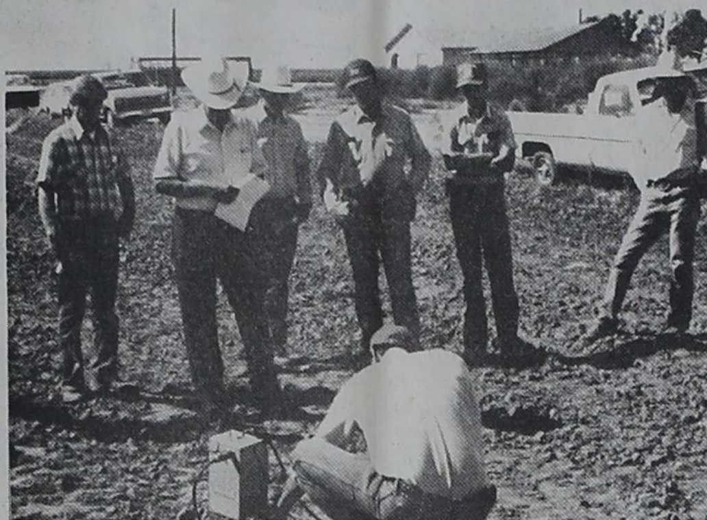
Jerry Walker, Civil Engineer with the Soil Conservation Service office in Amarillo, is explaining the use of the Neutron Probe. The Probe is used for soil moisture information at the depths of the root zones. The Probe is very active on moisture available to the growing plant.
