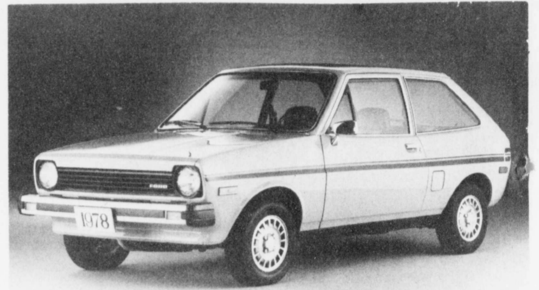
FORD'S POPULAR German-built mini-car, the Fiesta, is now available. Fiesta is powered by a performance-proven 1.6-liter Kent engine. Standard features include rack-and-pinion steering, MacPherson-strut front suspension, steel-belted radial tires, front disc brakes, front bucket seats and fold-down rear seat. It is available in one model—a three-door hatchback—with four trim levels: standard, Decor, Sport (shown here) and Ghia.
