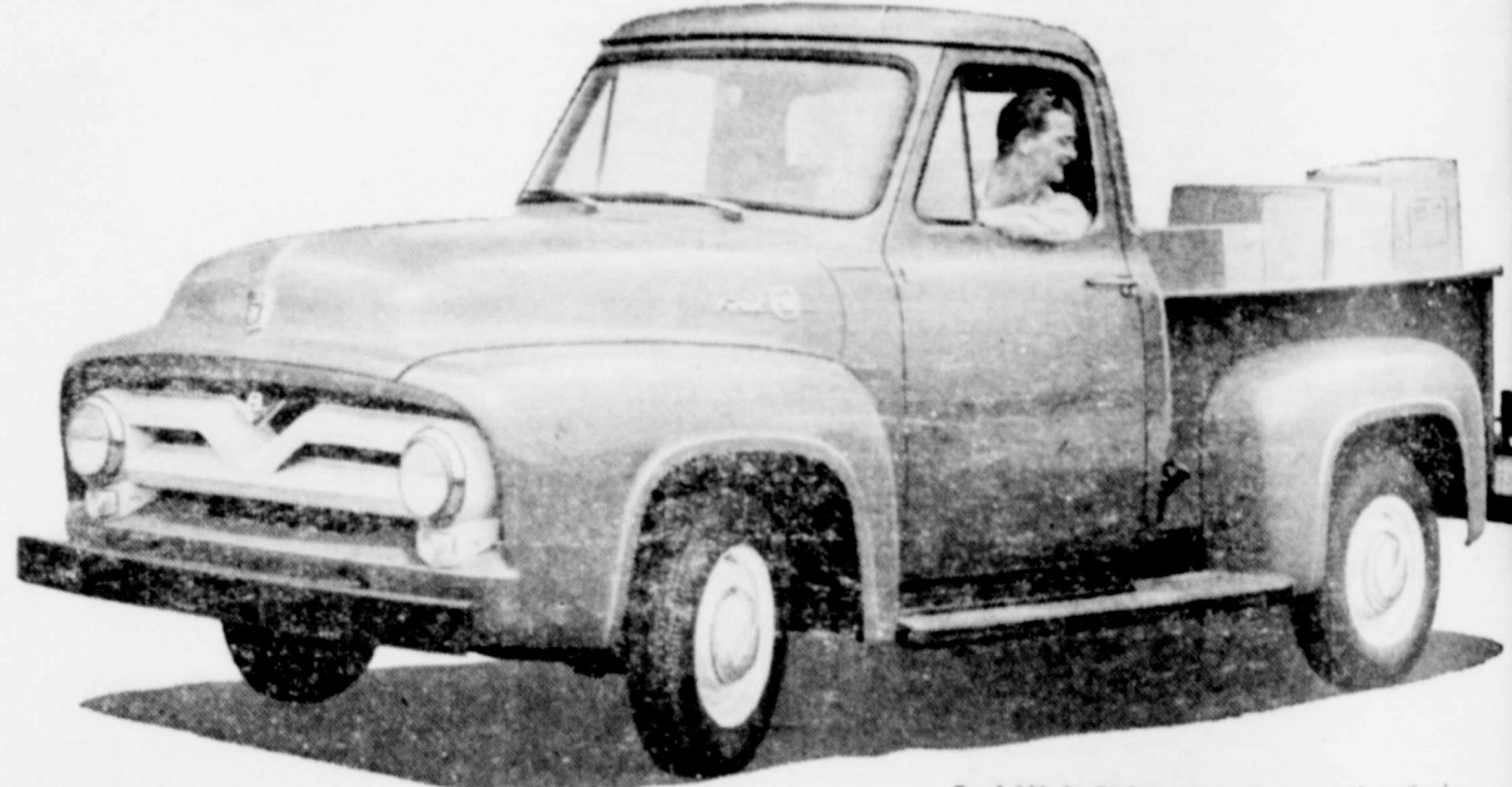
Ford 6 1/2-ft. Pickup gives choice of Short Stroke 132-h.p. V-8 or Short Stroke 118-h.p. Six. Tubeless tires standard. Fordomatic Drive and Power Brakes available at low extra cost. GVW 5,000 lbs.
