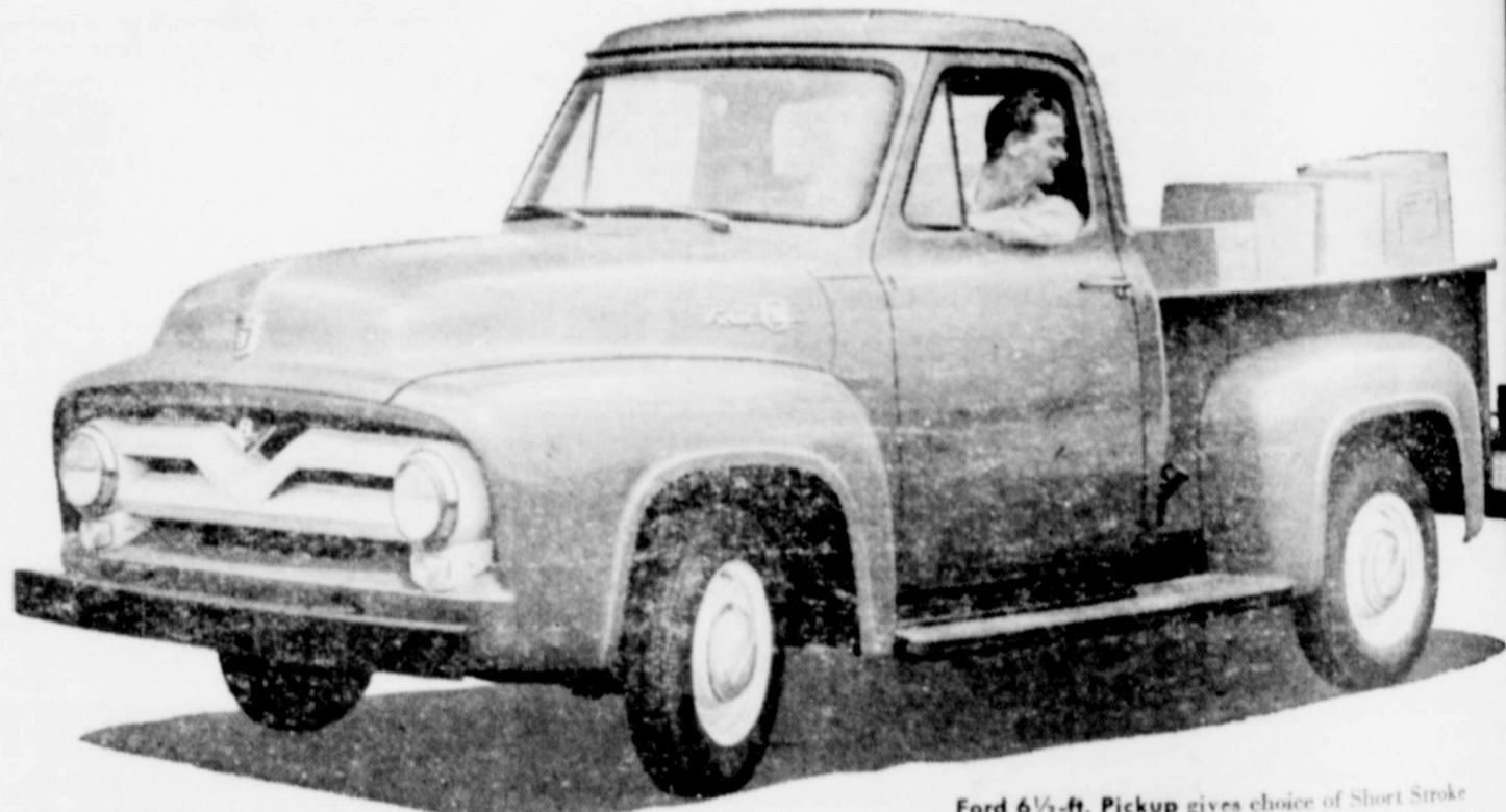
Ford 6 1/2-ft. Pickup gives choice of Short Stroke 132-h.p. V-8 or Short Stroke 118-h.p. Six. Tubelens tires standard. Fordomatic Drive and Power Brakes available at low extra cost. GVW 5,000 lbs.
