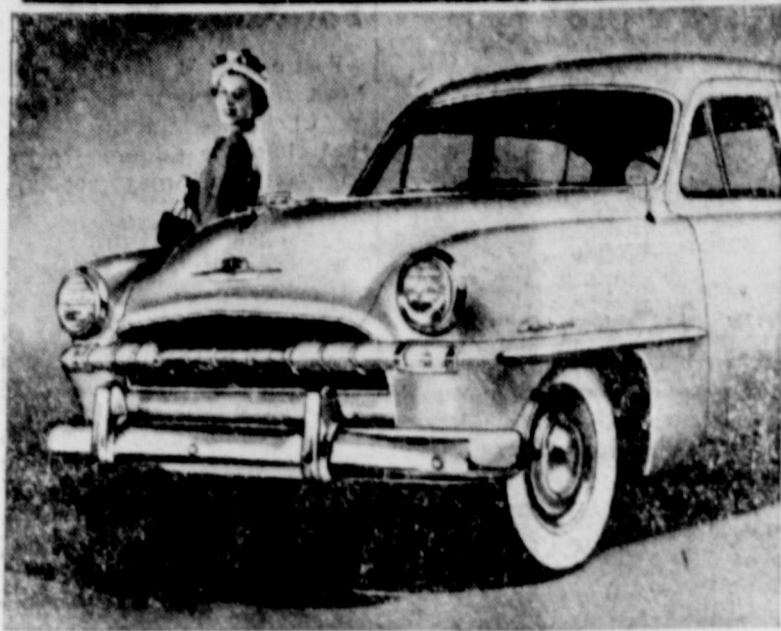
The distinctive grille of the 1953 Plymouth keynotes the new styling which carries through from bumper to bumper. The new models feature horizontal character lines that accentuate the ground hugging grace of the new streamlined styling. The softly rounded hood, sweeping out to the fenders, covers Plymouth's improved 100-horsepower engine with its 7.1 to 1 compression ratio. Note also the one-piece windshield with uniform curvature for minimum distortion and "Control Tower" visibility. It is available also in restful, heat-absorbing Solex tinted glass.
