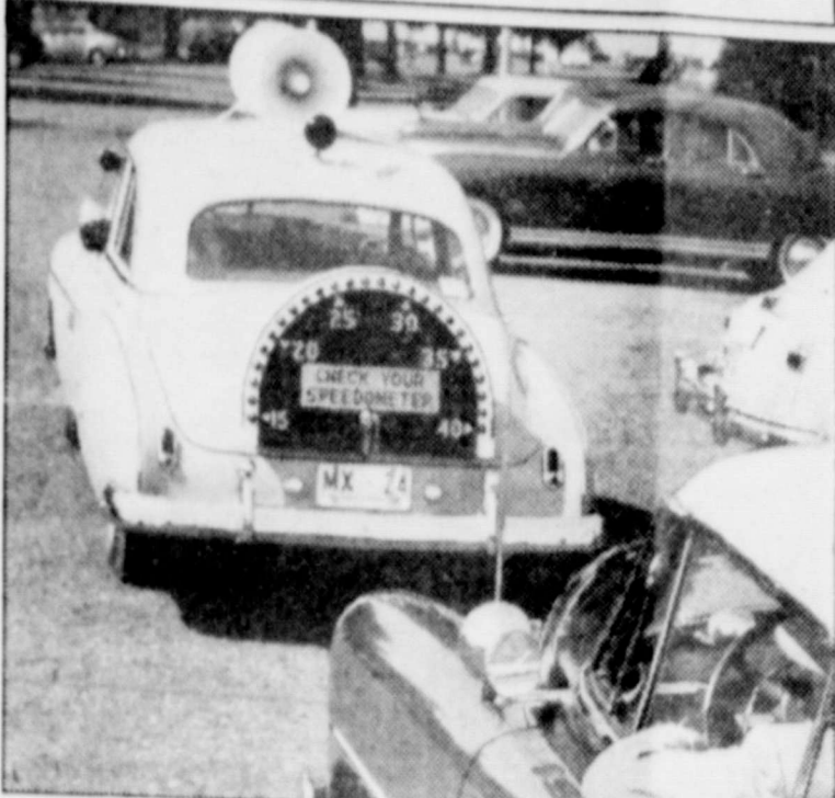
To make motorists conscious of speed limits, the Seattle, Wash. police department has put into operation a Powerglide Chevrolet with a precise speed check mounted at the rear.
