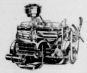
In Ford Series F-6 -- 110-Horsepower, 212 lbs.-H. Torque. le Ford Series F-6 COE - 106-Horsepower, 210 lbs. ft. Torque.
