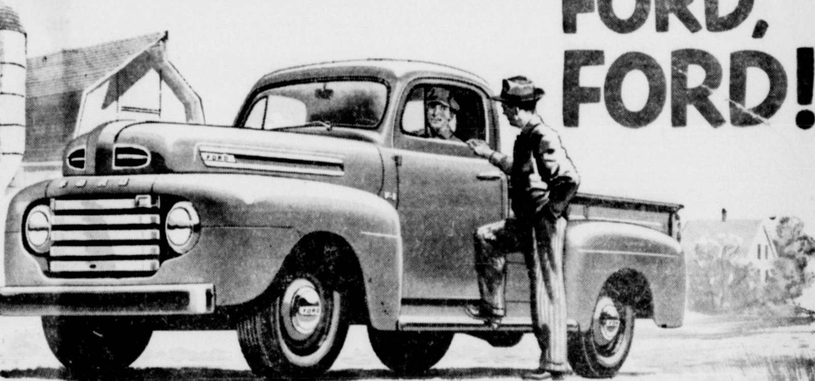
6 1/2-ft. Ford F-1 Pickup shown here. G.V.W. rating—4,700 lbs. Body capacity—45 cu. ft. Available with 95-h.p. Six or 100-h.p. V-8. One of over 175 models including 145-h.p. Big Jobs.
