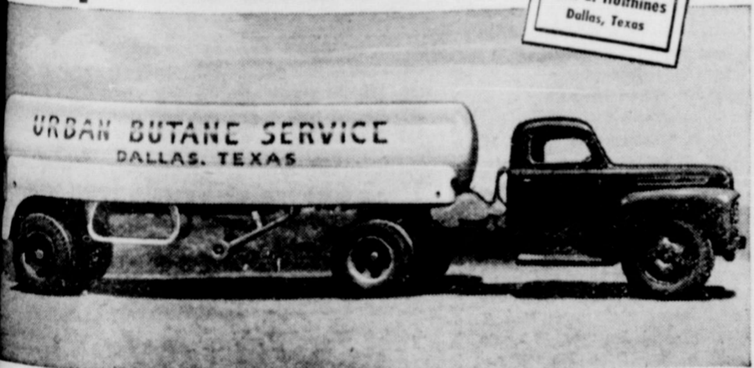
Ford Model F-7 BIG JOB shown has Gross Combination Weight rating of 35,000 lbs. as a tractor, Gross Vehicle Weight rating of 19,000 lbs.
