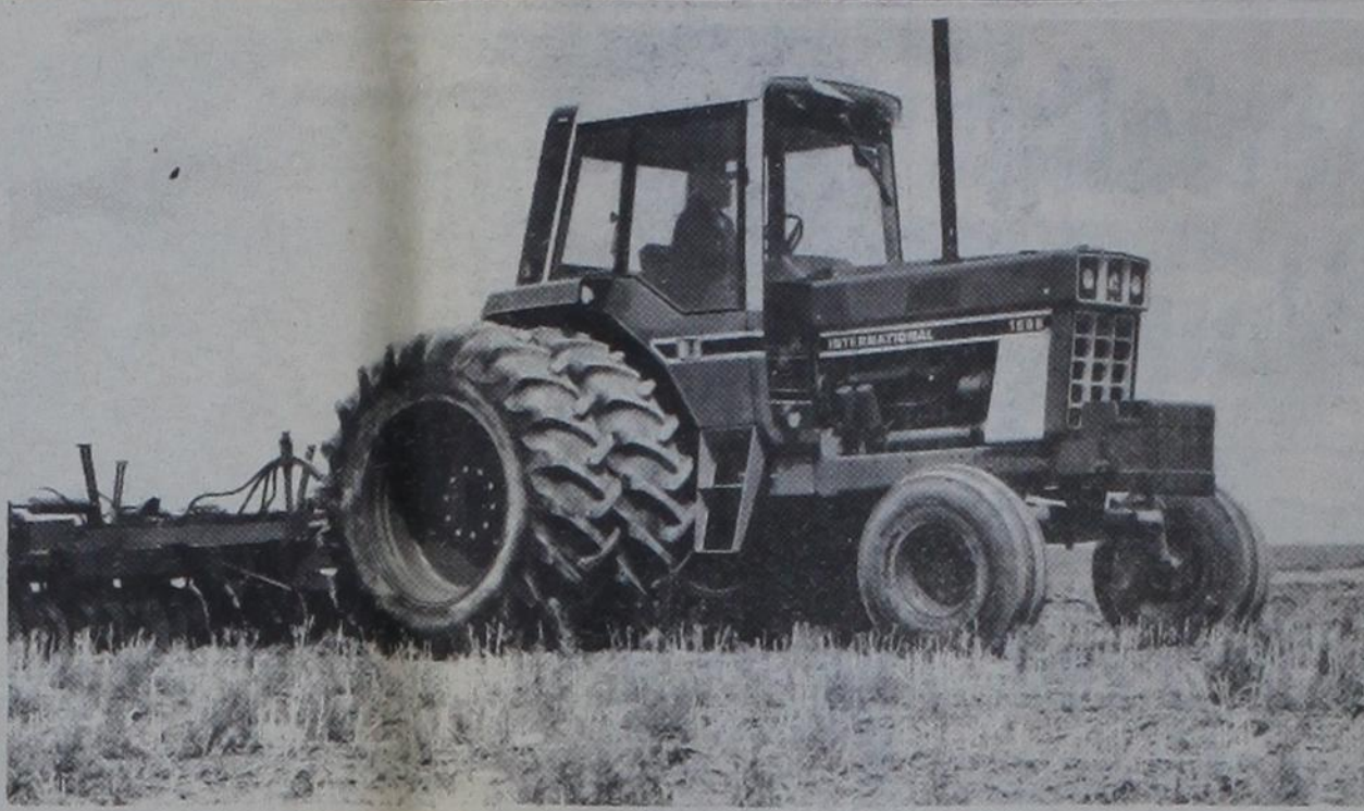
A 'CONTROL CENTER' CONCEPT is one of the main features of International Harvester's new Series 86 models for 1977. A departure from the add-on cab of the past, the air-tight "Control Center" is designed to provide maximum visibility and improved riding quality. It also accommodates aft-mounting of a larger fuel tank and molded auxiliary tanks on the left side of the tractor for a full day's continuous work. International Harvester's Series 86 "Pro-Ag" tractor lineup for 1977 was unveiled Saturday at Hays Implement Co. The model shown here is a 1586, with an estimated 160 PTO horsepower.
