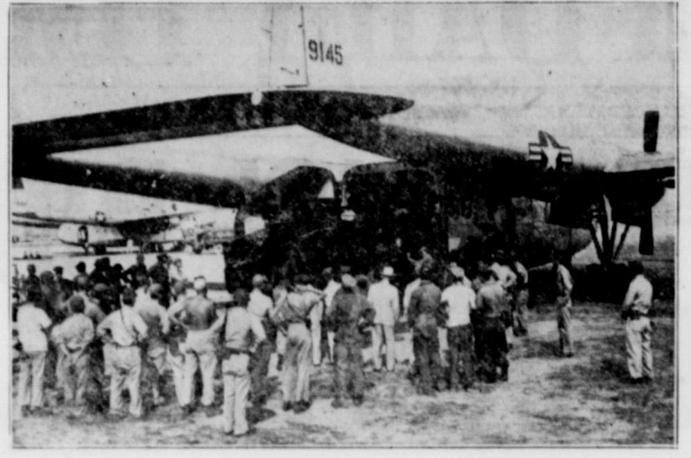
BIG TIME AIRLIFTING IN KOREA —How did the U. S. Armed Forces succeed in getting so many heavy trucks to the fighting front in Korea where ports are jammed and highways are few? The "flying boxcar" solved the problem. The "boxcar," you know, is the nickname of the big USAF C-119, a plane that carries a 15-ton cargo and swallows a 3 1/2-ton truck, whisking it in a space of minutes over mountains and out into the open close to the battle lines. Within an hour this truck, mounting the "boxcar" cargo, will carry needed supplies to GIs struggling against the enemy.
