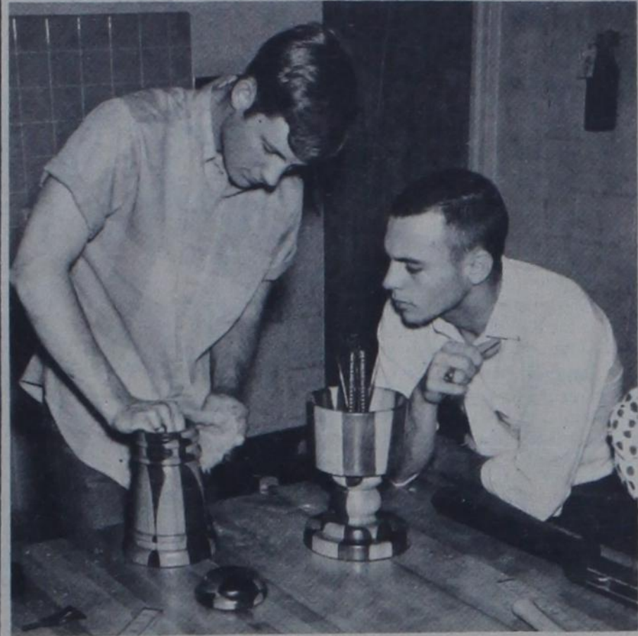
JOE BILL BUTLER, senior, uses pumice powder to put a shine on his decorative maple-and-walnut tankard. At right is Kenneth Oldham, a senior, with a maple-walnut laminated nut bowl. Both pieces were lathed from glued blocks.
