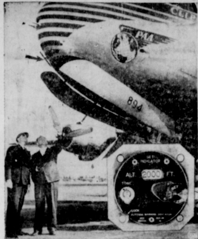
Two pilots examine the cigar-like forward antenna, arrow, of a new radar altimeter and warning device being installed on Pan American World Airways clippers. It sends out continuous radar impulses below and ahead of the plane, which are translated into feet-above-ground readings on a warning dial, inset, on the instrument panel. The device offers a virtually foolproof system to warn pilots of altitudes from 2000 down to 300 feet.
