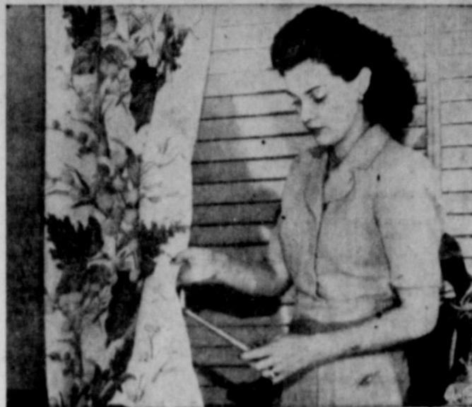
Paper drapes—costing less than a dollar a set—that will not burn are featured in New York's Curtain and Drapery Show. An open flame, like the candle in the picture, applied to these drapes, results only in a charred spot. They can be cleaned with a damp cloth.
