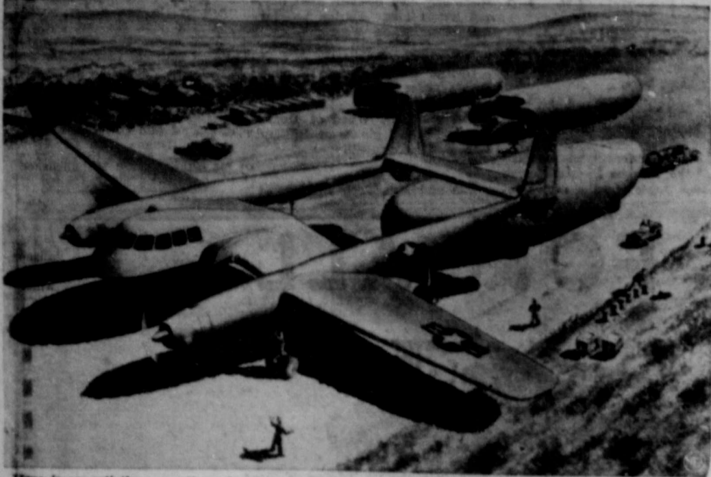
Here is an artist's conception of a new design for a flying boxcar with a detachable fuselage airplane to speed and facilitate handling of airborne cargo. The pod, or fuselage, could be loaded in advance of flight and attached to the plane before takeoff. The drawing above shows a pod being drawn away shortly after landing, while two other pods in background are being loaded for future flight. Now under consideration by the Air Materiel Command at Wright Field, Ohio, the design was drafted by the Fairchild Aircraft Division, Hagerstown, Md.
