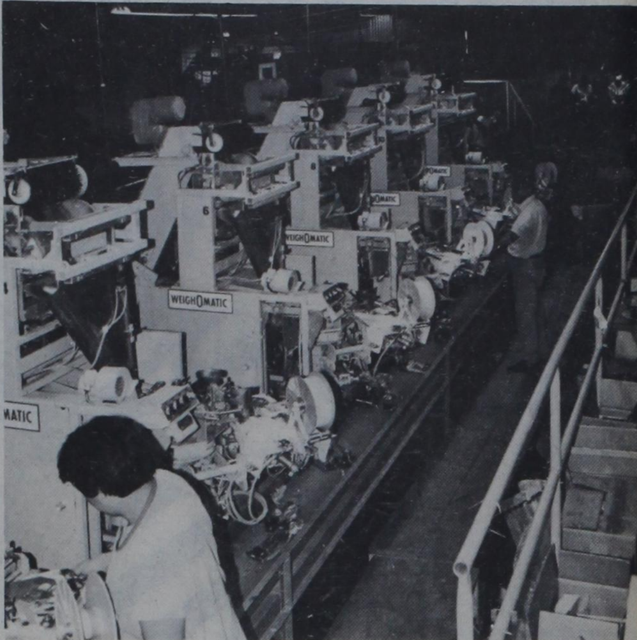
CARROTS are being automatically weighed and sacked this year at the processing plant of LaMantia, Cullum, Collier & Co. of Dimmitt, Inc. The plant has 12 of the new electronically controlled machines, which take washed and graded carrots off the conveyor and deliver one-pound tied bags, ready for the shelf. The LCC plant is processing 60 tons of carrots a day. Automated weighing and sacking is one of several innovations at the LCC plant this year.
