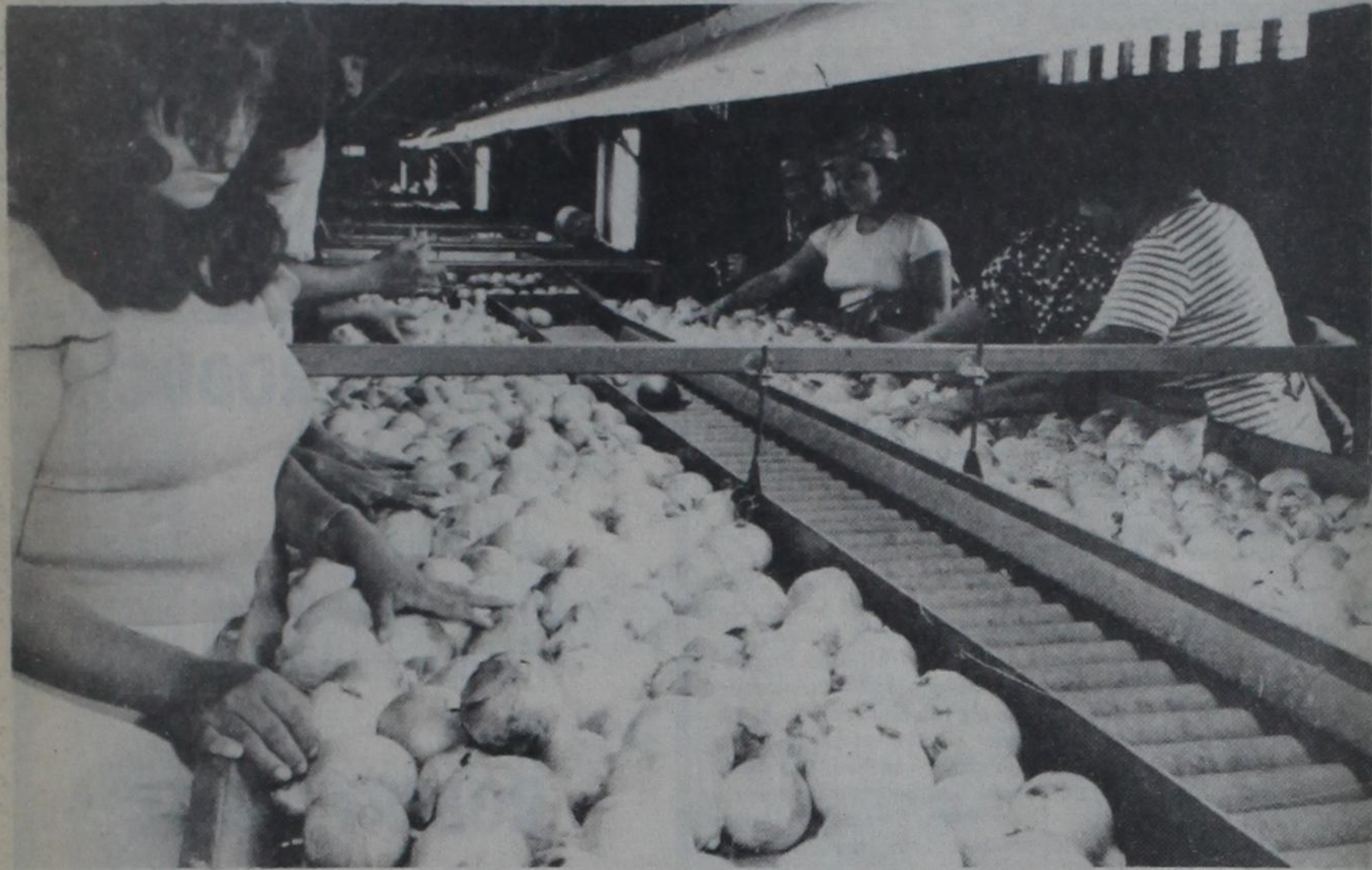
CASTRO COUNTY ONIONS flow along the grading line at the Dimmitt Vegetable Growers processing plant operated by La Mantia, Cullum, Collier & Co. The new onion processing machine—built to LCC's specifications at a cost of $90,000—slices the incoming onions before grading and enables the
