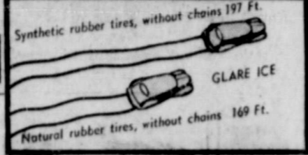
Synthetic rubber tires, without chains 197 Ft. Natural rubber tires, without chains 169 Ft.
