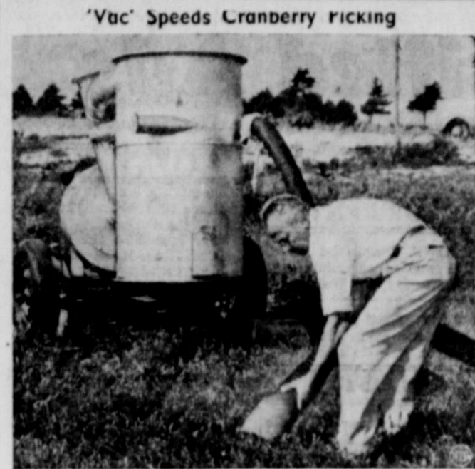
'Vac' Speeds Cranberry picking A farewell to the slow, laborious harvesting of cranberries by large numbers of workers crawling across a field is seen in this "vacuum cleaner" mechanical picker, pictured being tested at Hanson, Mass., by Antone Lenari, Cranberry Cannery, Inc., engineer. By vacuum, berries are sucked off vines into hose, from which they go into the big container, which is rubber-lined to prevent bruising. The machine was developed by growers in collaboration with the U. S. Rubber Co.
