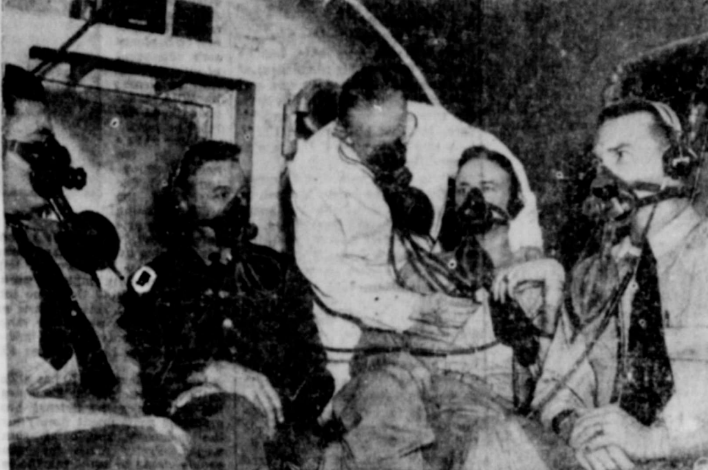
Not only is World War II being fought largely in the air, but it is being fought at higher altitudes. U. S. Army technicians are developing equipment and men to perform at top efficiency in atmosphere above 25,000 feet. Above, Dr. J. W. Helm examines heart reactions of flyers in 40-foot pressure test chambers, under conditions simulating ascent to 35,000 feet, at Wright Field, Dayton, O. Seated, left to right: Capt. Curtis Low; Cap. E. J. Tracy; Lieut. F. A. McNaughton, and Lieut. C. R. Bond
