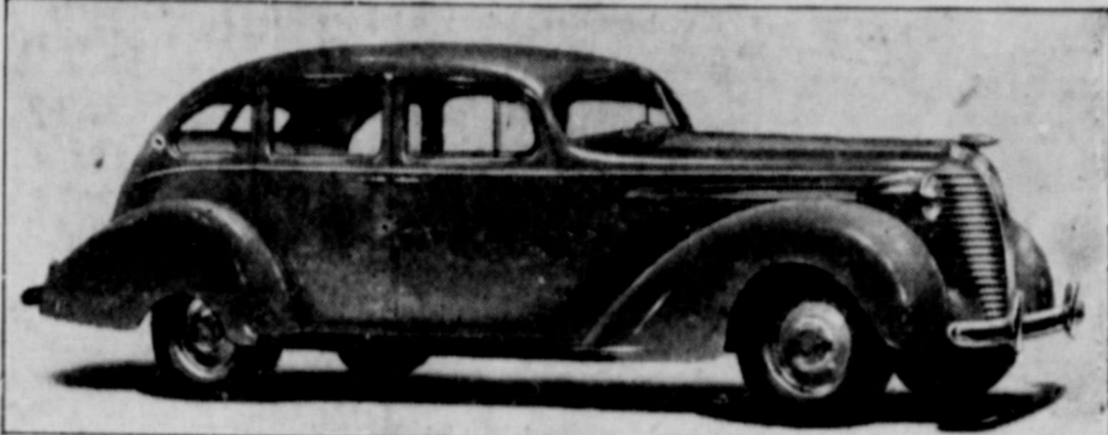
The Hudson Terraplane Sedan in the Deluxe series is on 117-inch wheelbase and has a 96-horsepower engine. The Hudson Super Terraplane, on the same wheelbase, has five additional horsepower.
