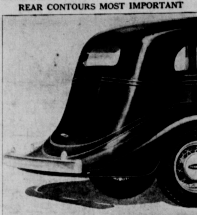
Streamlining efficiency in motor car design depends largely on rear-end contours. Hudson engineers learned from wind-tunnel tests and, in consequence, the 1934 Terraplanes and Hudsons sweep to the rear as shown here, with no outside-mounted tire to break the flowing lines. The car front contributes only 25 per cent to streamlining possibilities, and the rear and sides 75 per cent.
