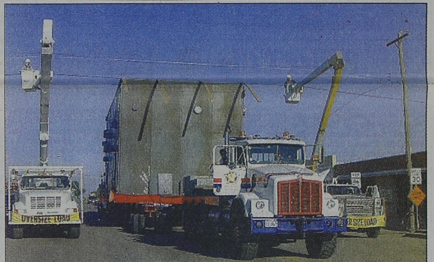
IT'S BIG AND IT'S HEAVY —A cold box being shipped from Tucson, Ariz., to Borger came through Dimmitt Tuesday morning. Used to "turn gases into liquid," the box was 25 feet tall and 60 feet long and
