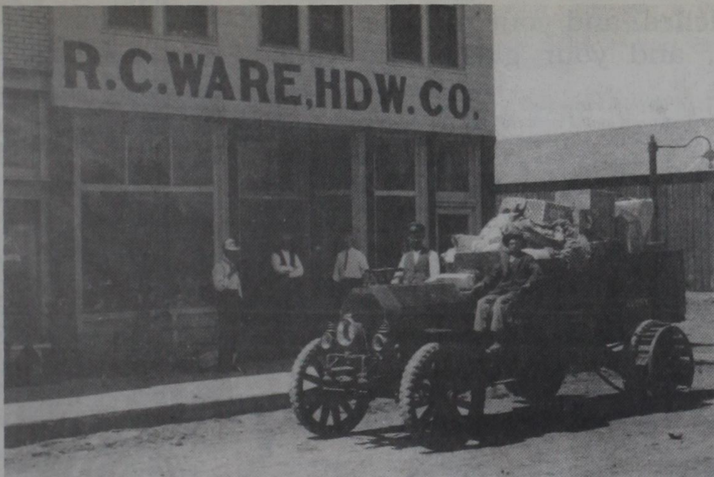
M. E. Cleavinger Sr. (shown here with his son, Jess, in 1913) hauled freight between Springlake and Plainview in the early days in this Avery truck. Note blade-type metal mud grips on rear wheels.
