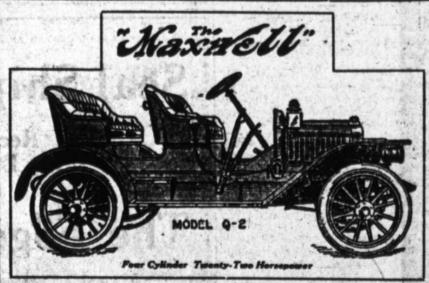
MOTOR 3 3-4x4 inches. Ignition Double, Magneto and Battery. Transmission Sliding Gear, three speeds forward and reverse. WHEELBASE 93 inches, WHEELS 30 inches. TIRES 30x3 1-2, COLOR, blue with black leather upholstery.
