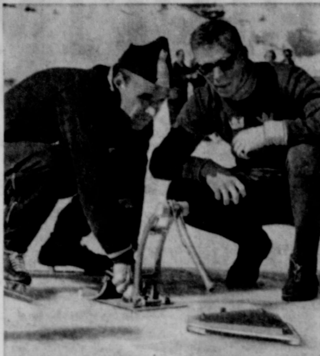
GLIDEMETER —Speed-skating competitors at Squaw Valley, Calif., get together on one thing. They both want to know: "How slick is the ice?" Gadget, pictured, is a miniature, spring-propelled sled. Distance it glides is compared against performance figures on lee of other rinks. Gadget belongs to Russian assistant team manager Ivan Anikarov, left. Watching the track is Swedish speed skater Hans Wilhelmsson.
