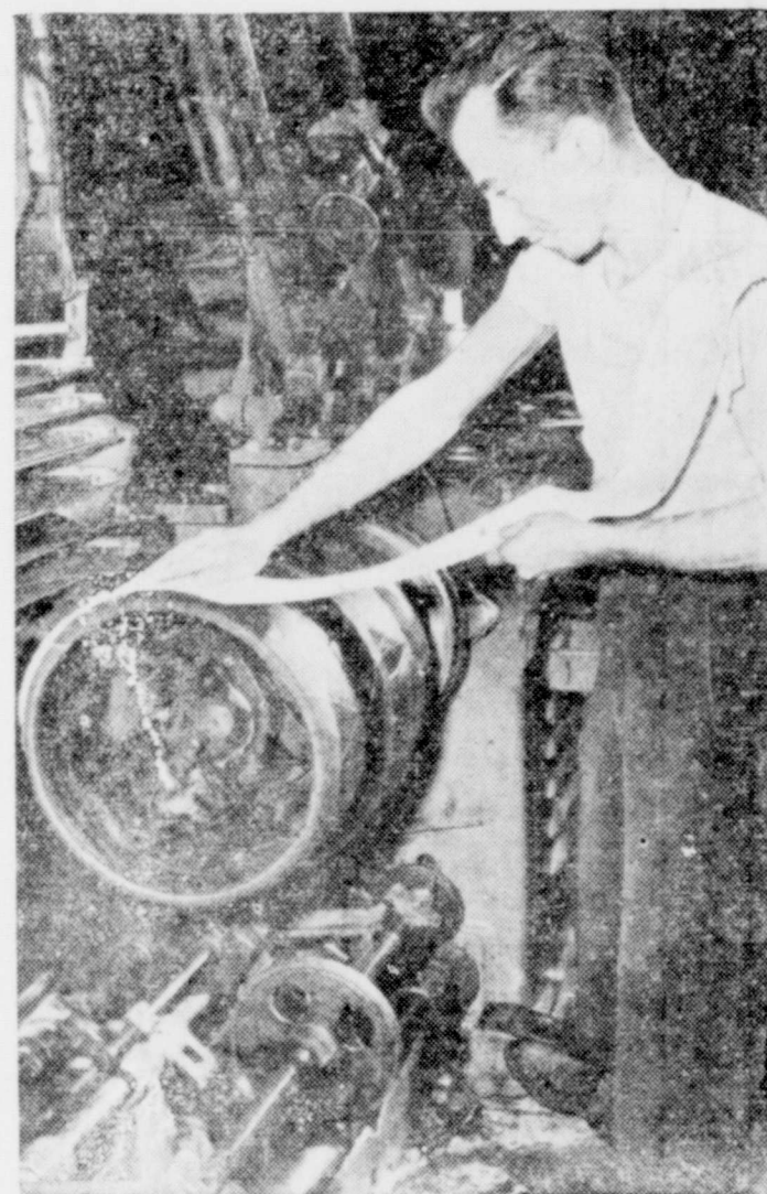
WHITE SIDEWALL TIRES AGAIN—Discontinued at the outbreak of the war, the manufacture of white sidewall tires is resumed. Here Joe Chesko, Goodrich employee, applies the white strip to tire. CPA regulations allow company 50 a month.
