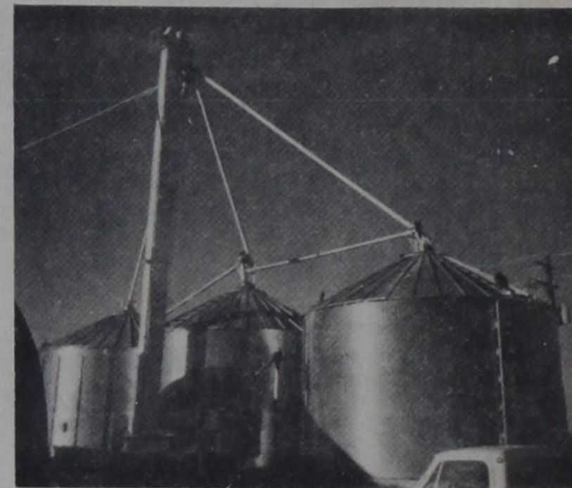
THREE-BIN CONTINUOUS CORN DRYER ON THE FARM OF ALLAN WEBB
