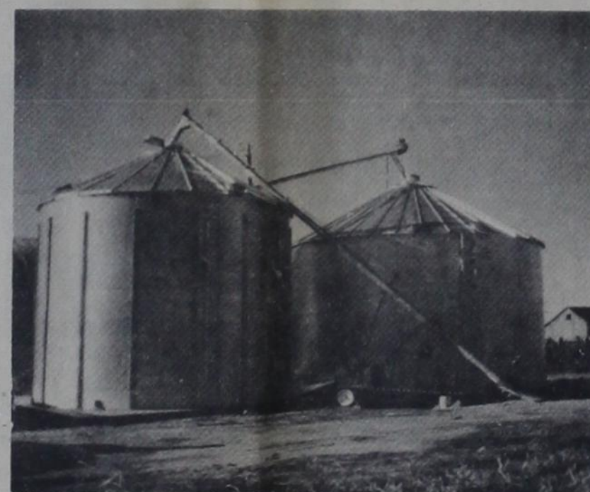
TWO-BIN CONTINUOUS FLOW CORN DRYER ON THE FARM OF R. A. AXTELL
