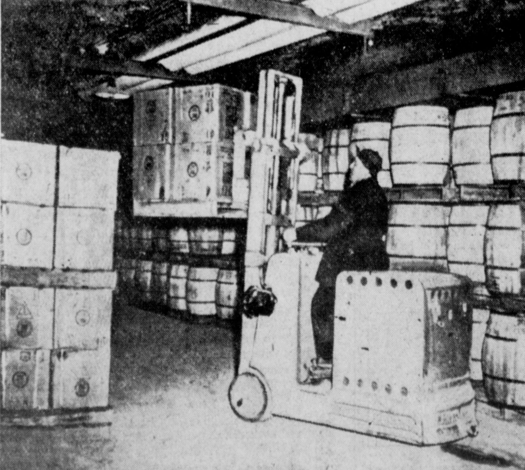
NATURAL COOLER—The world's largest natural cooler on a single floor, located in a 75-year-old limestone mine at Atchison, Kans., stores provisions for UNRRA. Here a hoist lifts eight cases of food into place. Capacity of the cooler is 92,000 tons.
