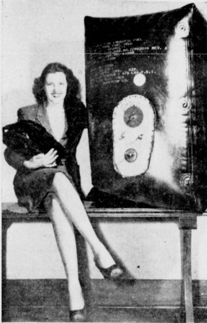
SAVED MANY AIRMEN'S LIVES—A peacetime version of the bullet-sealing fuel cells that saved many airmen from going down in flames, is this 50-gallon gas tank made of nylon and synthetic rubber. Virginia Summers of the Goodrich Co., Akron, holds the folded-up version that is no bigger than first base.
